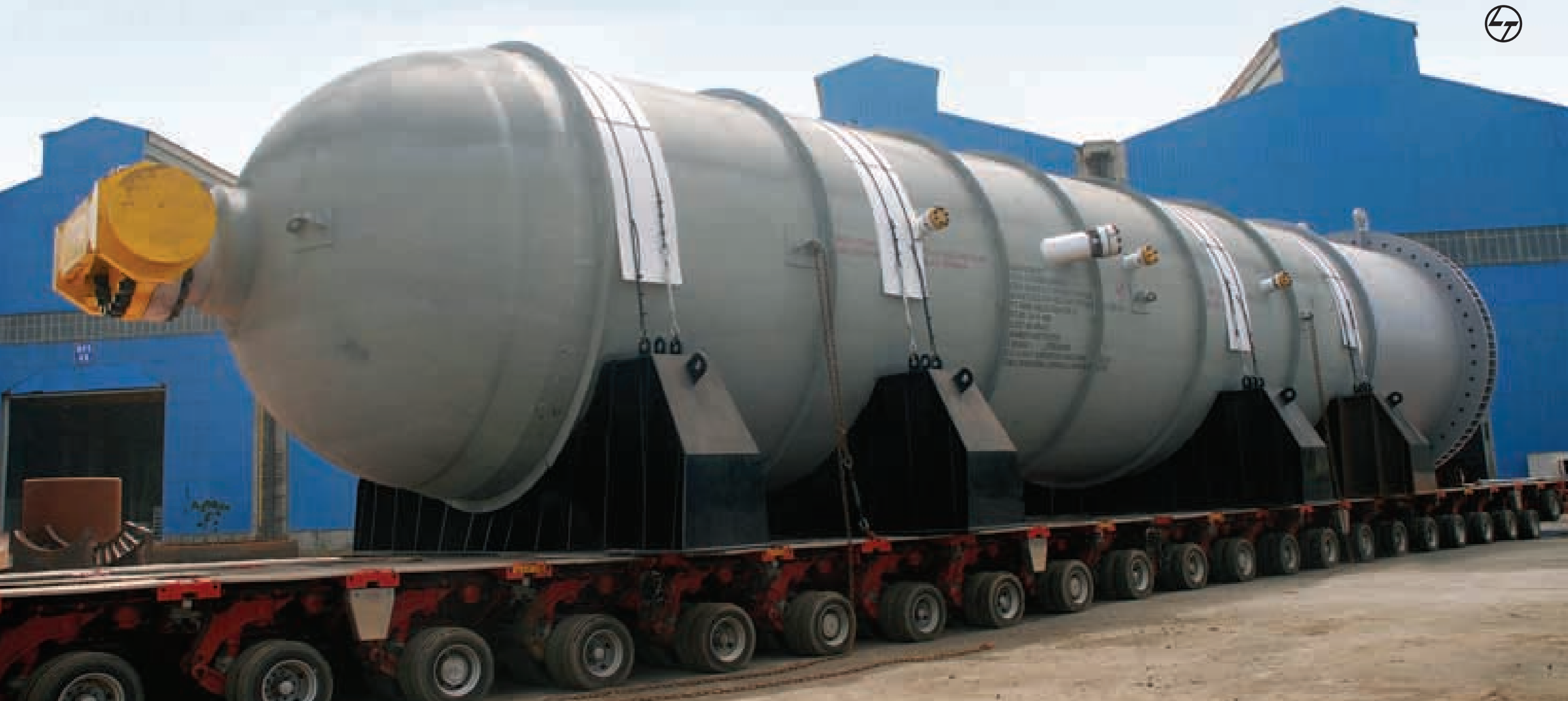
Chrome-Molybdenum-Vanadium Hydrocracker Reactor with 300mm-thick walls, weighing 1000MT, being exported to Greece from Hazira Manufacturing Complex. L&T offers a comprehensive range of critical equipment and systems, including high-pressure heat exchangers, to the hydrocarbon sector worldwide.
