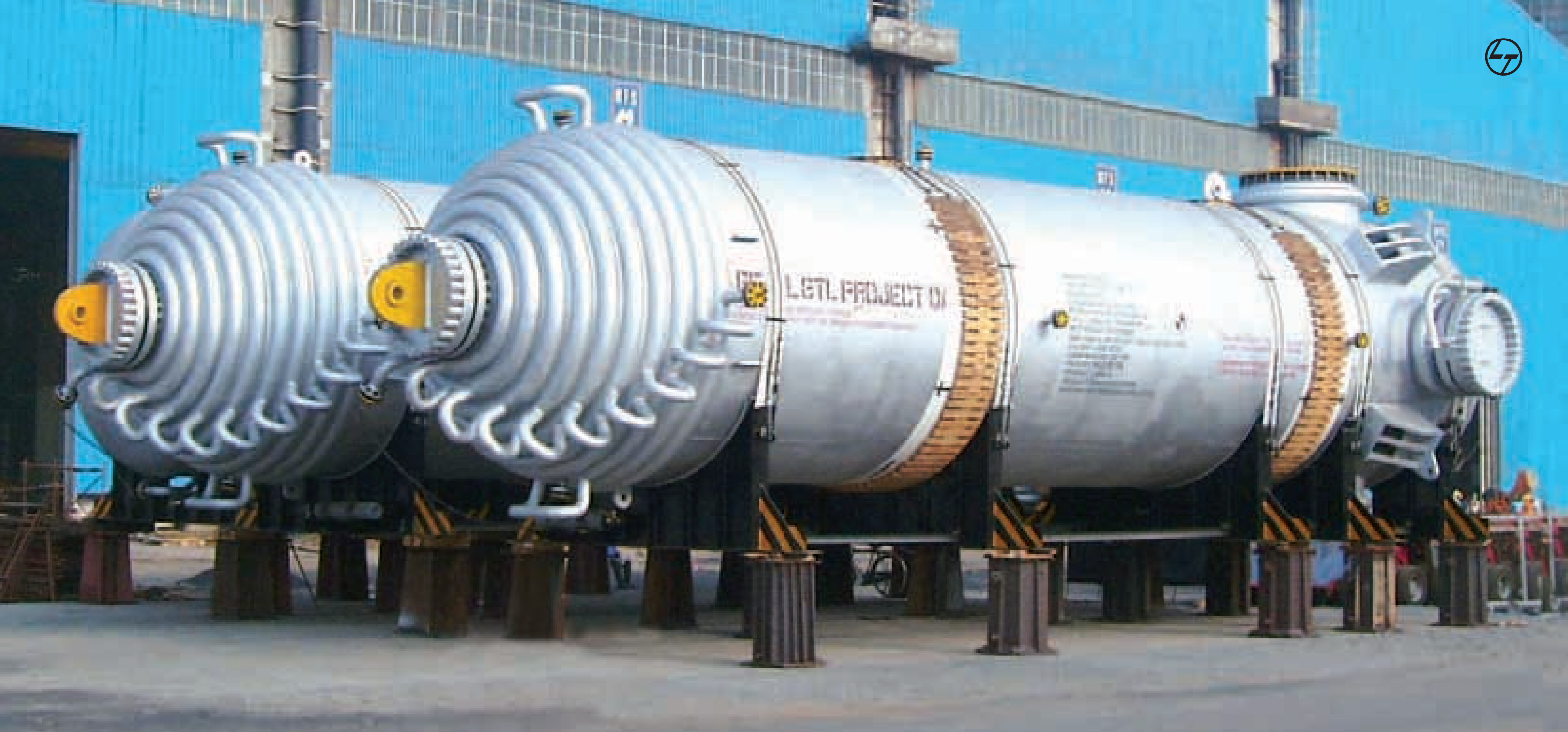
SGP Reactors for Qatar Shell gas-to-liquid project ready for despatch. L&T's Hazira Manufacturing Complex has its own roll-on-roll-off jetty, offering direct access to the Arabian Sea.
