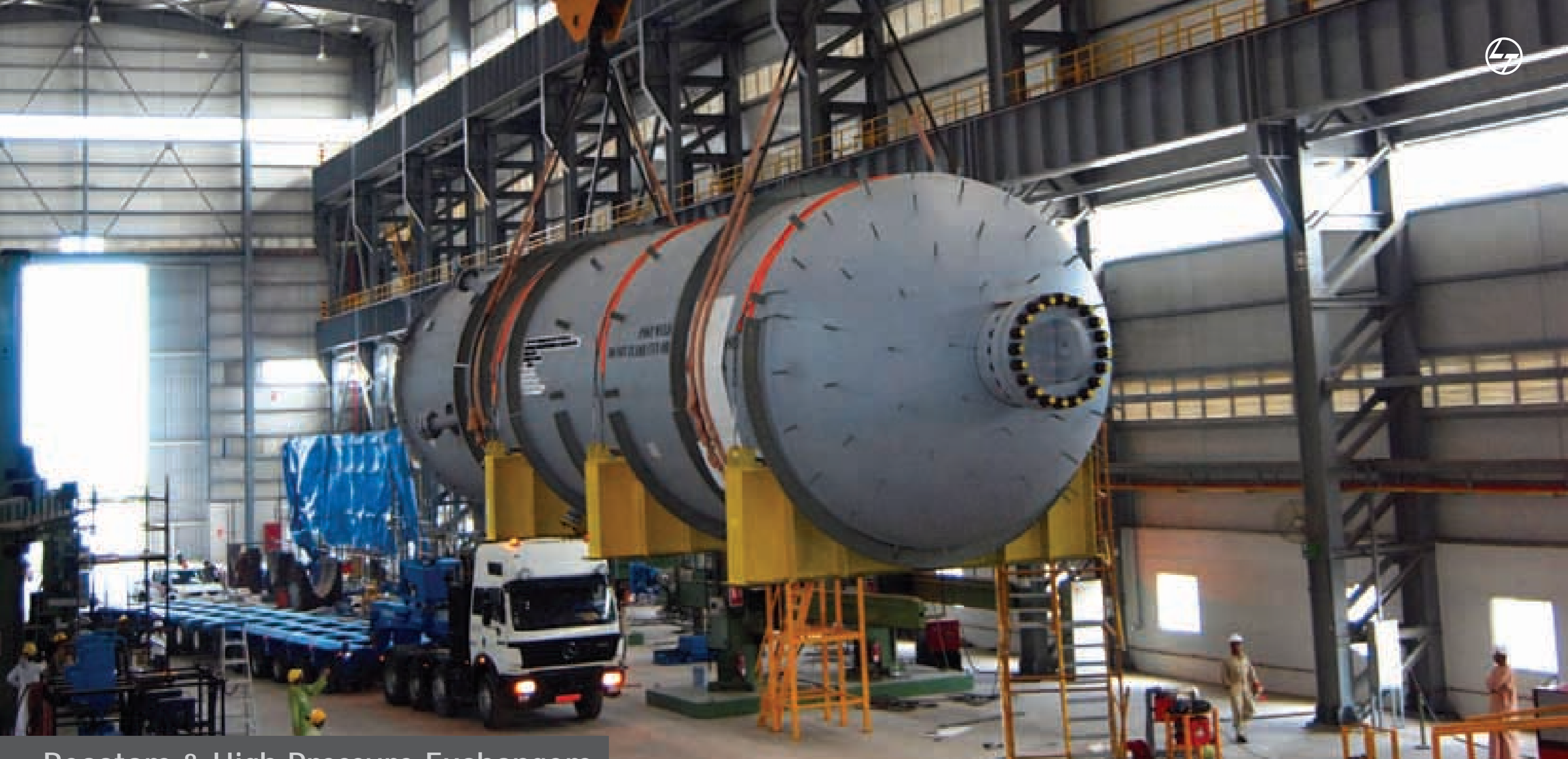
Cr-Mo HDS reactor manufactured at L&T's Sohar complex in Oman. The complex includes a captive jetty with direct access to the Gulf of Oman.
