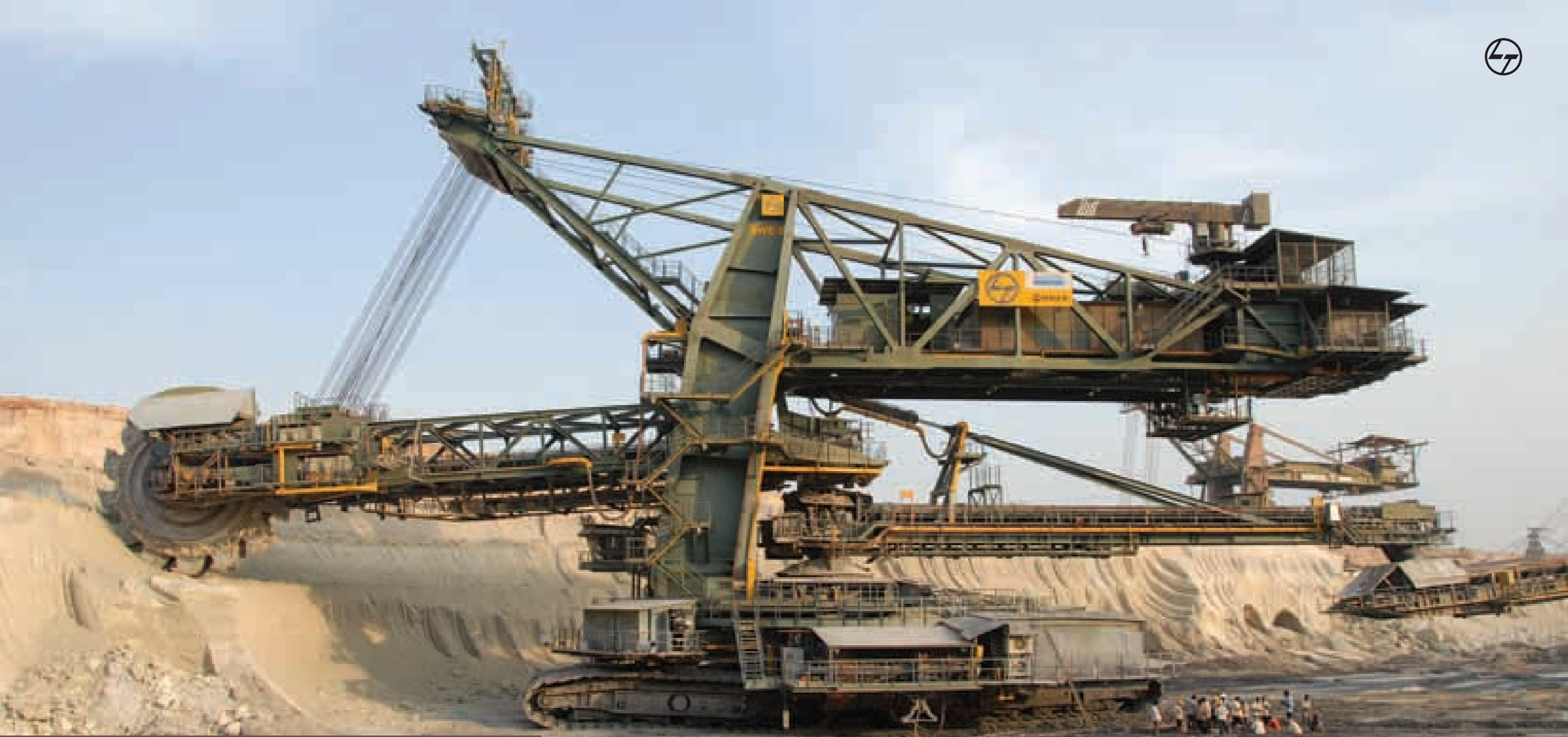
2730 cu.m.per hour capacity bucket-wheel excavator manufactured and supplied by L&T for the Mines II Expansion Project of Neyveli Lignite Corporation. L&T's product profile in this segment includes wagon loading systems, stockyard equipment and port-handling equipment and conveyor systems.
