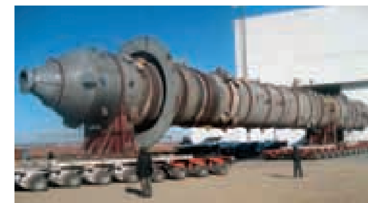
Section of a coal gasifier - one of many supplied to China. L&T has manufactured and supplied the world's largest coal gasifier to China.
